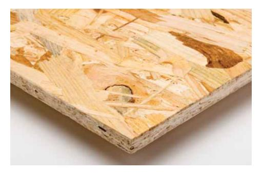
The extra layer in Kronospan OSB3 provides the same excellent structural and durability characteristics of OSB2, but with the additional benefit of resistance to humidity.
